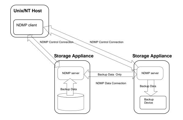
Figure 2 - NDMP client backing up data on a tape-less file server to another file server with a local tape device
