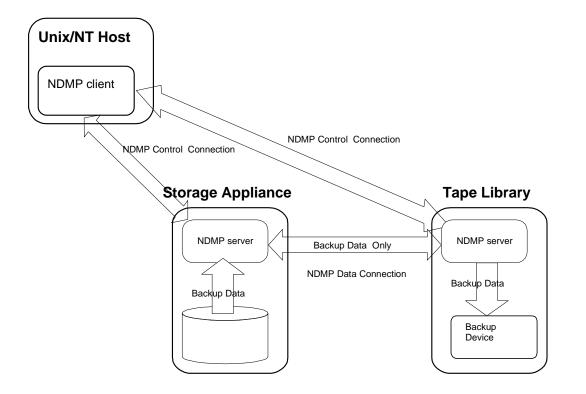
Figure 3 - NDMP client backing up data on a file server to a network attached tape library
